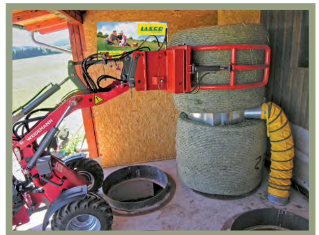
The distribution hose supplies the second row with additional drying air.
