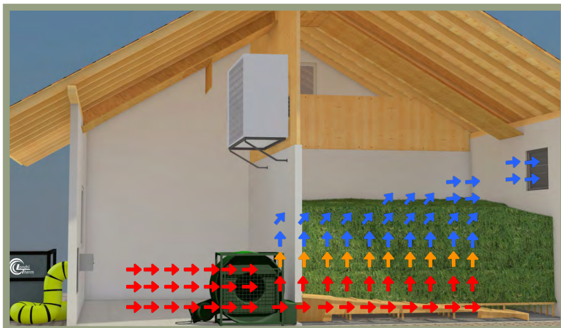
Scheme of a drying plant with LandriTherm warm air heater.
