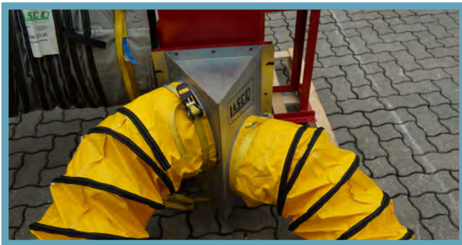
Consistent drying due to double blow-in paths.
