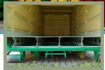
Consistent drying due to double blow-in paths.
