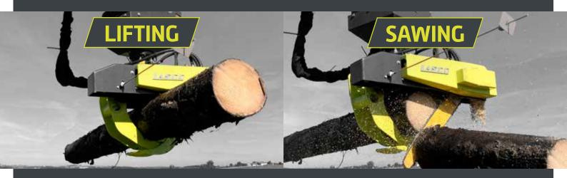
The LACombi DUOSCORP combines timber gripper and harvester saw. It chops up wood quickly and effort-lessly. Not only agricultural and forestry businesses, but also municipal operations appreciate the swift sorting and cutting to length of tree trunks with diameters up to 60 cm. Felling of problematic trees is another application area for the DUOSCORP. It can easily remove individual standing trees with a diameter of 20 cm over the remaining stock.
