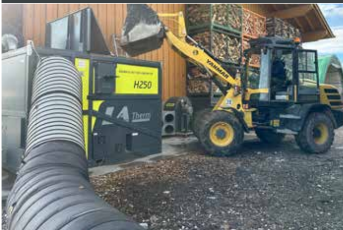
Simple loading of an H250 with a wheel loader. The H250 is connected directly to two drying containers.
