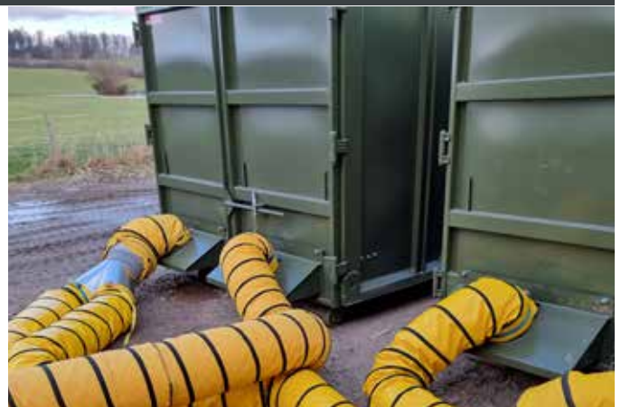
Heat distribution made easy. The drying air enters the drying container effortlessly via warm air hoses.
